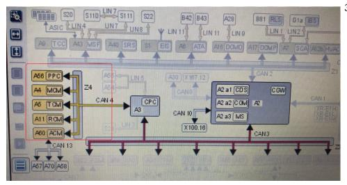
3. Connect Board Control CAN module to the CAN4 bus. Connection is possible in different places: star point Z4 at cab, or under front grille, or direct on ACM socket. Find +15 PWR and GND using multimetr.
