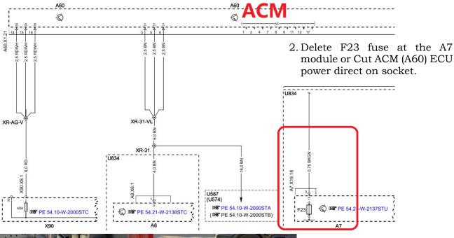
Or CUT power direct on the ACM socket
